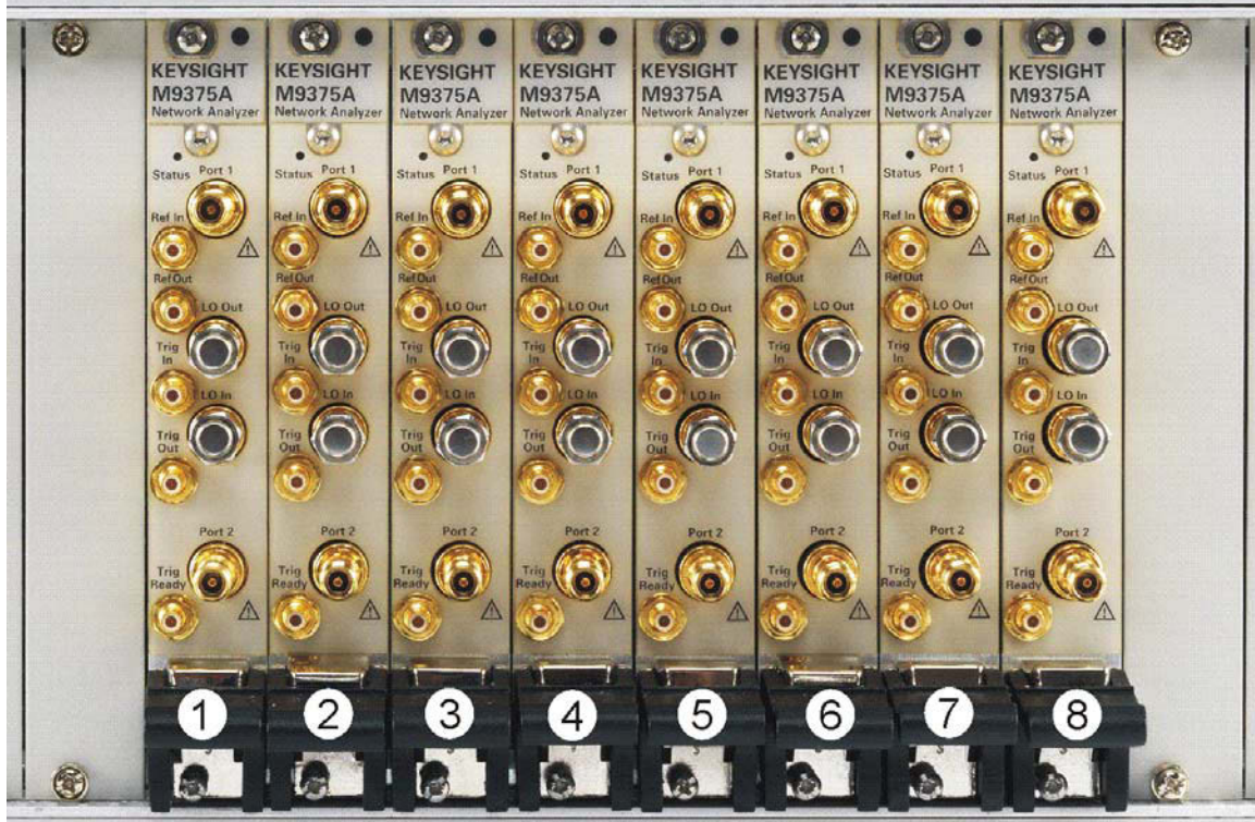
Figure 1-5 50 Ohm Loads Installed on the Network Analyzer Modules
